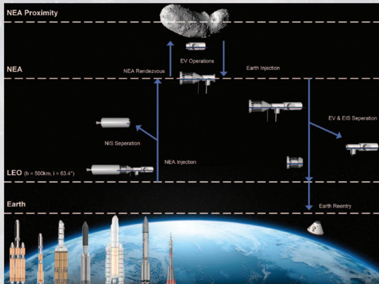
the assembly is 91 days. Time between two launches is set to 14 days in order to provide enough time for the assembly process in space. The assembling orbit has a declination of  $i=63.4^\circ$ .
