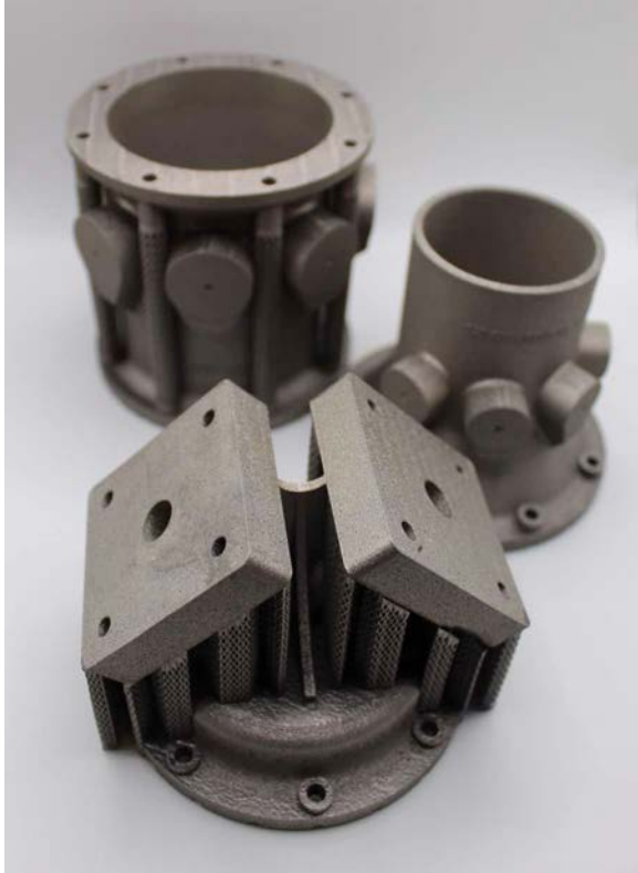
Figure 8. Mark 1 chamber pressure shell parts in Inconel 718 (throat fuel film cooling manifold not implemented)
