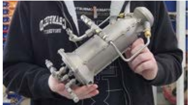
Figure 7. Mark 0 water cooled monolithic engine chamber manufactured using ALM in Inconel 718.
