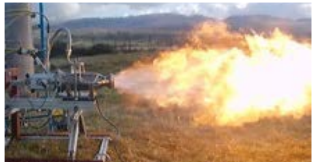
Figure 8. Hot fire ignition test of Mark 0 engine chamber at Snowdonia Aerospace Centre
