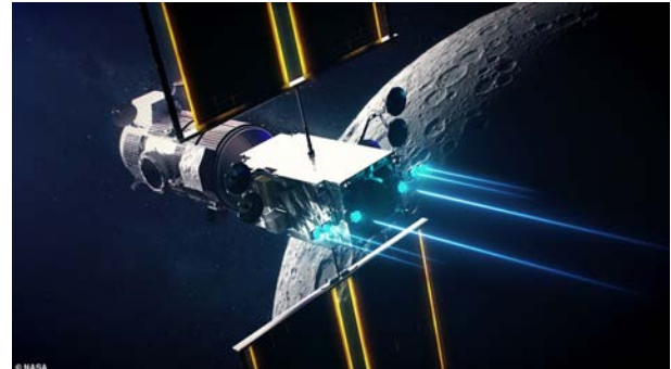
Figure 1. Artists rendering of Lunar Gateway Space Station and its orbit maintenance electric propulsion (Image credit: NASA).
