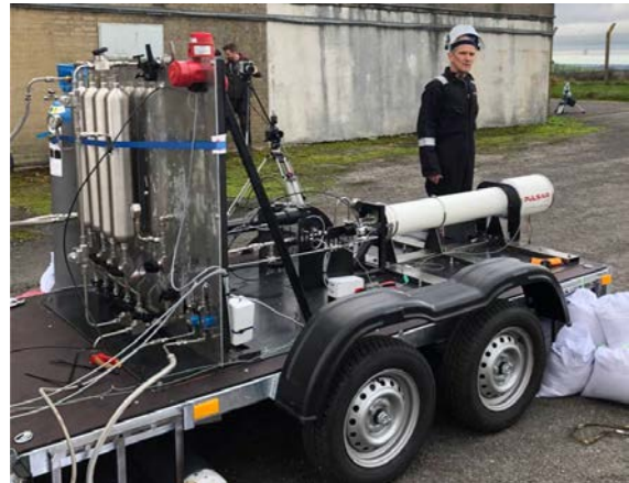
Figure 10. Portable engine test rig (hybrid rocket example). (Image Credit: Pulsar Fusion)
