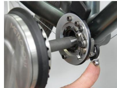
**Step 12:** Install Drive side (Right) crankarm ① by sliding the spindle through the drive side (right) BB cup, through the BB shell, and out the Non-Drive side (left) BB cup.
