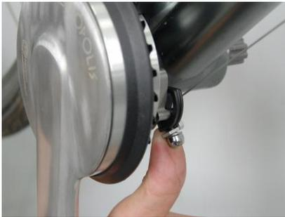
**Step 13:** Release the cable arm.
