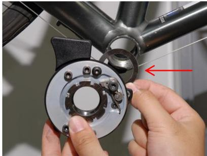
**Step 2:** Place the Drive side (Right) BB cup ③ through the Control plate sub-assembly ⑤ and the seal washer "D" as shown in the photo. Thread the BB cup ③ into the right side of the BB shell. Keep the black Inboard chain guard in the top (12 o'clock) position.
