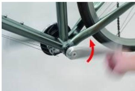
**Step 20:** Spin the crankset in normal direction and operating the shifter to check if the whole system works properly.
