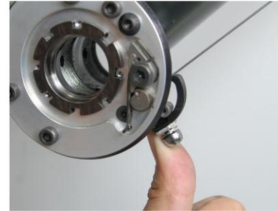
**Step 11:** Use a finger to move the cable arm (at the back of Control plate sub-assembly) to full forward position, and hold until step 12 is completed.
