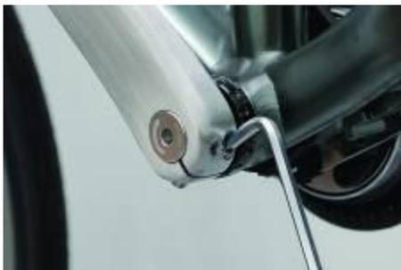
**Step 15:** Use the 5mm hex wrench "c" to tighten the pinch bolts of the Non-drive side (Left) crank arm ② to a torque value of 10.8 to 14.7Nm.
