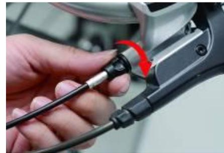
**Step 16:** Screw the front shifter barrel adjuster completely inward to reserve the adjustment range as much as possible. Check the shifter is at the lowest position possible. Usually #1 on most gear indicators.
