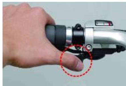
**Step 19:** Ensure the shift lever can be easily operated between two lowest gear positions (#1 & #2 on most gear indicators).
