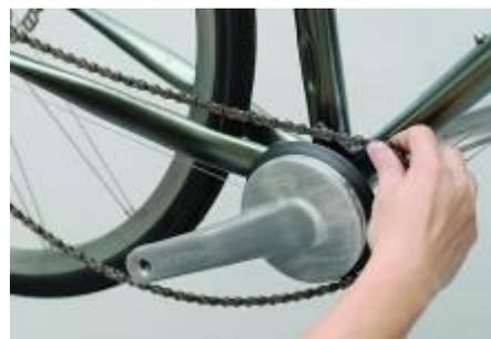
**Step 22:** Install the chain and pedals on the crankset. Follow pedal manufacturer's instructions.
