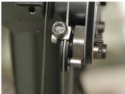
**Step 18:** Ensure that the shifter cable is seated in the groove of the cable arm, and fixed tightly. Loosen cable pinch bolt and re-tighten if shifter cable is not seated in the groove.
