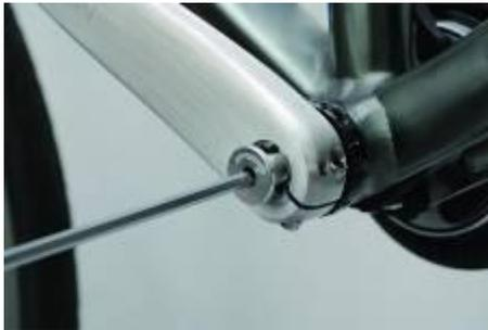
**Step 14:** Install the Non-drive side (Left) crank arm ② on the BB spindle, ensuring that the crank arms are 180° opposite of each other. Apply medium strength threadlocker to the spindle bolt "B." Use the 5mm hex wrench "c" to tighten the spindle bolt to a torque value of **0.7 to 1.5Nm**.
