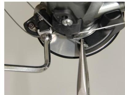
**Step 17:** Thread the cable down to the cable arm, and install it through the cable pinch plate. Tighten the cable pinch bolt with 4mm hex wrench to a torque value of 5 to 7 N-m.
