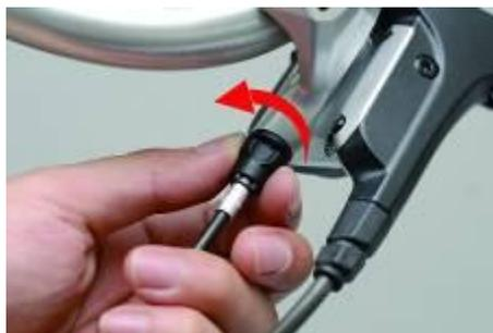
**Step 21:** Check shifting function while spinning the crankset. If there is a clattering noise during the upshift or in the second gear position, screw the barrel adjuster on the shifter outwards while continuously spinning the crankset until the noise disappears.
