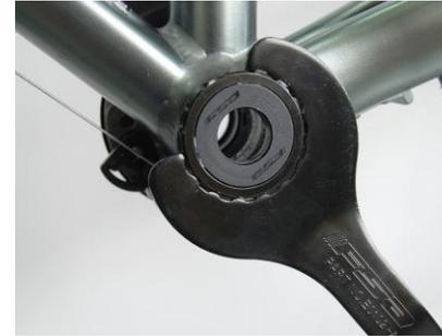
**Step 10:** Install the Non drive side (Left) BB cup with waterproof sleeve ④. Use the an external bottom bracket wrench "a" to tighten it to a torque value of 40 to 50Nm.
