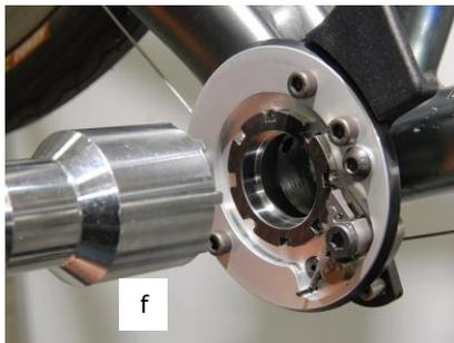
**Step 3:** Use the "f." Socket BB-18 wrench to thread the Drive side (Right) BB cup completely into the BB shell. Use very little torque. **DO NOT** fully tighten.
