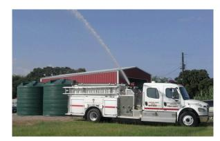
Each water plant can provide 50-gpm of agricultural grade water to keep the tanks filled. The high-pressure pumps can fill a 1,000-gallon fire engine in just four minutes! That's fast! These new water plants at stations #2 and #3 on LCR 750 and FM 3371, respectively, join the water plant at the main fire station on FM 937. All together the WLLVFD and EDS#2 have 57,000-gallons of firefighting water available to meet fire emergencies in the south county.
