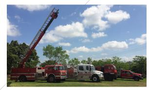
This picture includes two attack engines on the left and two brush trucks on the right. The one on the far right is a rescue vehicle that is equipped with bumper sprayers, and hand lines with a 500-gallon water tank in the back. The second from the right is our large, rough country, brush truck with a 750-gallon tank and two hand lines. It too has bumper sprayers which allow the vehicle driver to "roll" along a fire's front as firefighters in the rear pour water on the flames from 1" hand lines.
