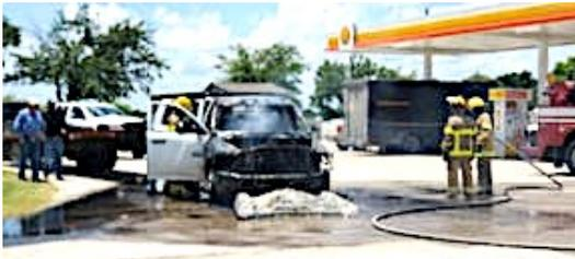
and pry open the driver door. A lithium battery within the console continued to burn, requiring further efforts to extinguish the fire. Firefighters conducted a survey of the burnt vehicle using a thermal imager to confirm the fire was out and the temperatures were cooling.
