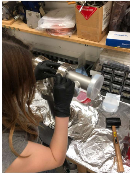
Figure 7: Tightening Reducing T-Flange to Valve Connection
