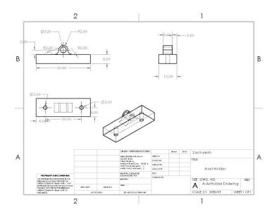
B. 6V Motor Holder (printed 2, one for each motor):
