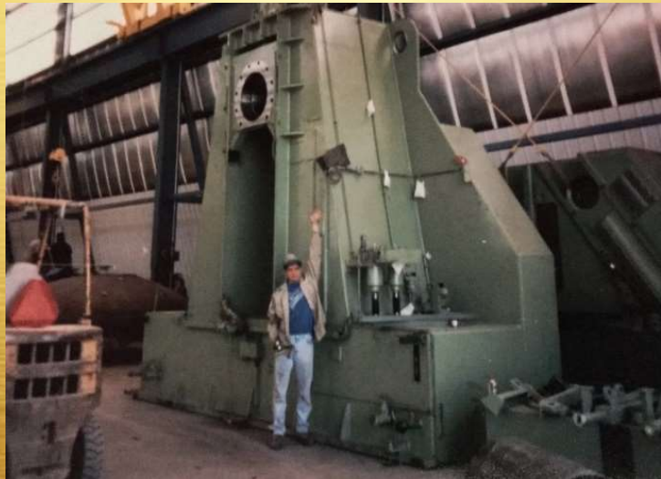
Hauseler Roller 5.75" Thick, 10' W, 4' to 20'OD
