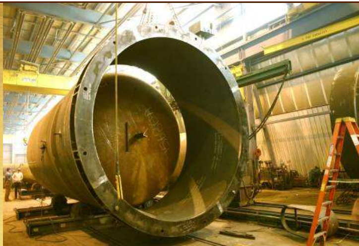
Pullmax Roller 1.75" Thick, 10' W, 17" to 15' OD
