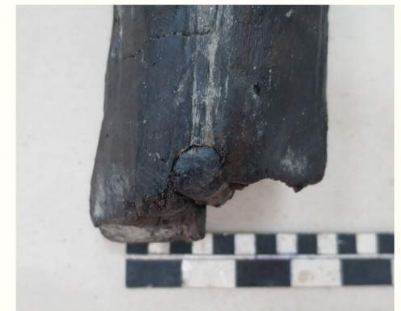
Pinned scarf joint in a frame timber.
