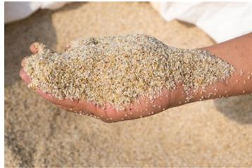
Conigliaro Industries received a sample of the material and quickly determined that the material was clean and suitable as a concrete aggregate additive. The filter sand was blended with standard concrete sand as well as recycled aggregates such as crushed concrete, brick, porcelain and glass.
