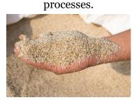
Conigliaro Industries received a sample of the material and quickly determined that the material was clean and suitable as a concrete aggregate additive. The filter sand was blended with standard concrete sand as well as recycled aggregates such as crushed concrete, brick, porcelain and glass.
