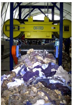
WHAT'S LEFT: Shredded cloth and foam roll down a conveyor belt at Conigliaro Industries in Framingham, Mass., after metal and wood are separated at the mattress recycling facility.
