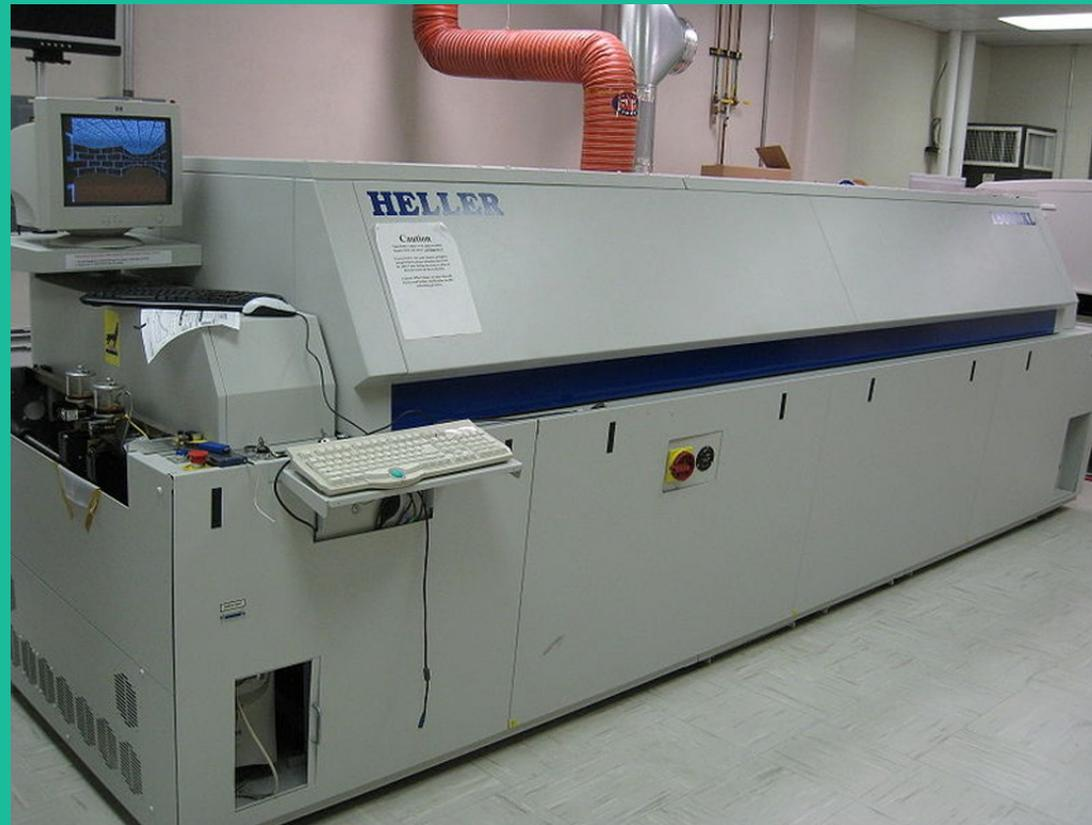
Reflow oven can match/far exceed capacity of pick and place machine.
