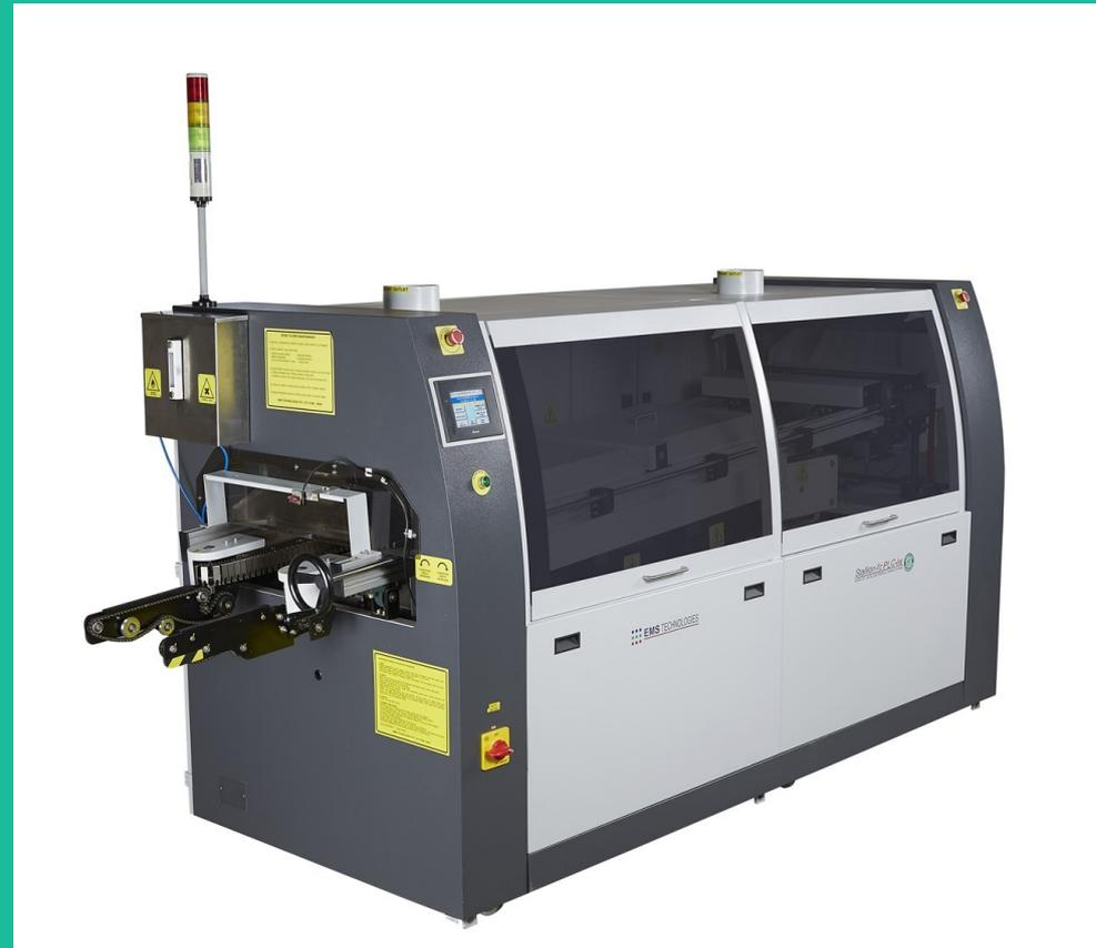
For PCBs with SMD and Thruhole components, we need a wave soldering machine. One machine can easily process matching components for PCBs processed on pick and place machine.
