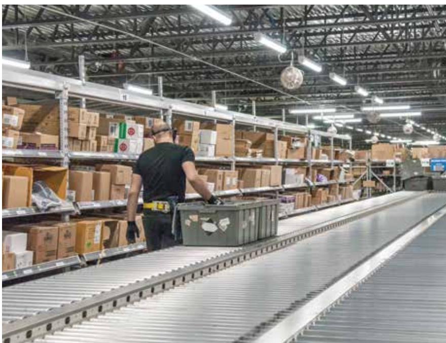
Items are picked to totes in pick modules (bottom) and then conveyed to a cross-belt sortation system for order consolidation (top).
