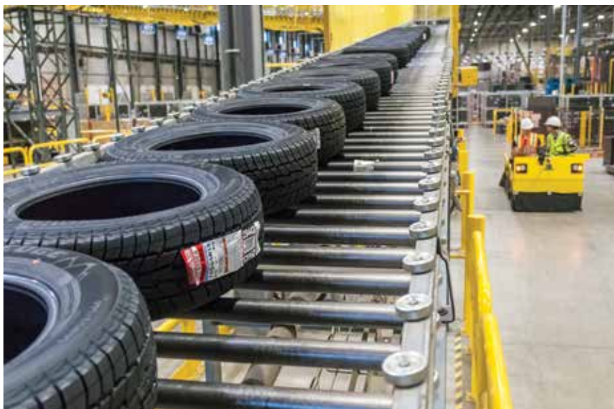
Newly received tires are conveyed to the gantry robotic tire handling system.
