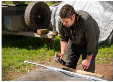
For really hard-to-get-at places and for componentry such as bolts, nuts and springs, spray-on zinc coatings are hard to beat. The mixture is usually 93 per cent zinc and it can be welded or powder coated once it has set.
