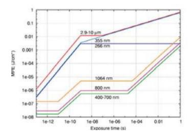
Maximum permissible exposure (MPE) at the cornea for a collimated laser beam
