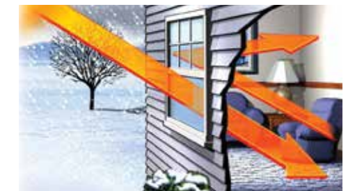
Winter Energy Savings: Low-E insulating glass reduces heat loss by reflecting warm air back into your home.
