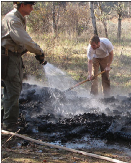
If you want to save the biochar, you need some water for quenching. A light mist and some shovel work will do the job.
