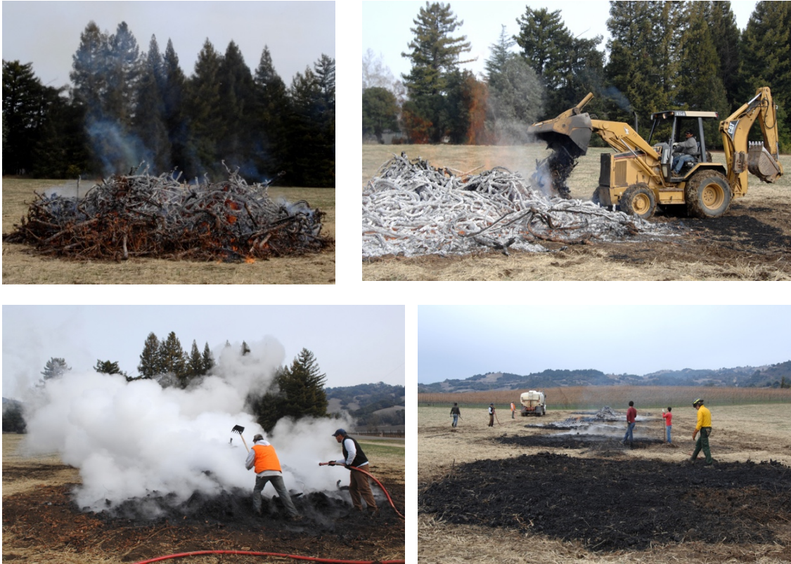
Figure 7. Once the pile collapses, it is time to tend and consolidate it. Quenching uses a combination of water and spreading to cool the char. If the char is not spread out, residual heat can evaporate all the water and re-ignite the char. Photos: Raymond Baltar/Sonoma Biochar Initiative.
