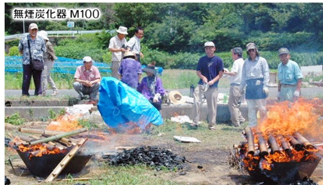
Figure 10. Left: A pit kiln used in Hawaii to produce commercial quantities of biochar (photo: Josiah Hunt, Pacific Biochar). Above: a cone-shaped kiln available from the Moki company chars bamboo in Japan.
