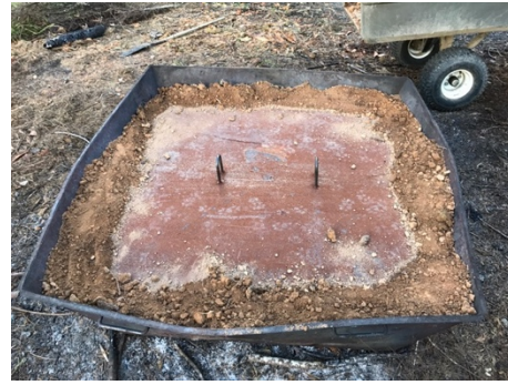
Figure 9. When the Flame Cap Kiln is full of glowing coals, it is time to quench it. Flood quenching is most effective, but dry quenching can also be used. Here (above) a thin sheet steel lid is placed on top of the hot coals and sealed with dirt or clay. Photos: WBA
