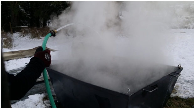
Figure 9. When the Flame Cap Kiln is full of glowing coals, it is time to quench it. Flood quenching is most effective, but dry quenching can also be used. Here (above) a thin sheet steel lid is placed on top of the hot coals and sealed with dirt or clay. Photos: WBA
