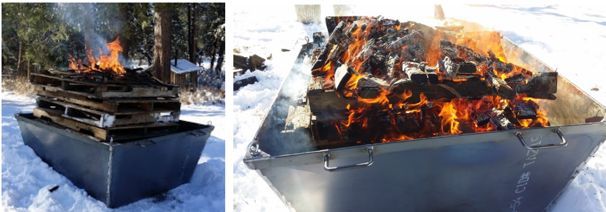
Figure 8. The Oregon Kiln making biochar on a small goat dairy for use in the barn. Start the Flame Cap Kiln with a top-lit rick. Once the initial charge burns down, start adding new material in layers. The flame front moves down as the rick burns down, and then moves back up as the container is filled. Photos: WBA
