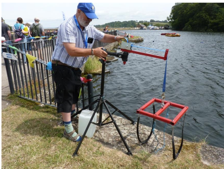
Our Derek demonstrates his own design of model launch gear, lashed to the metal barrier and weighted by a water-filled canister
