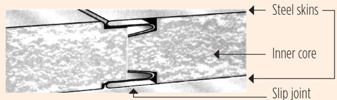
Figure 1: Typical Insulated Sandwich Panel
