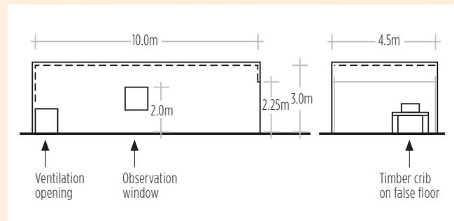
Figure 2: LPS 1181 Room Test (source<sup>14</sup>)
