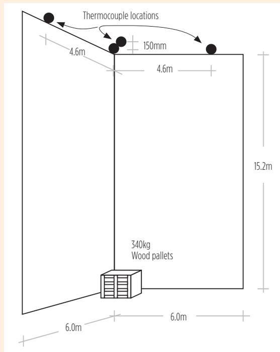
Figure 3: 50ft Corner Test (source<sup>18</sup>)
