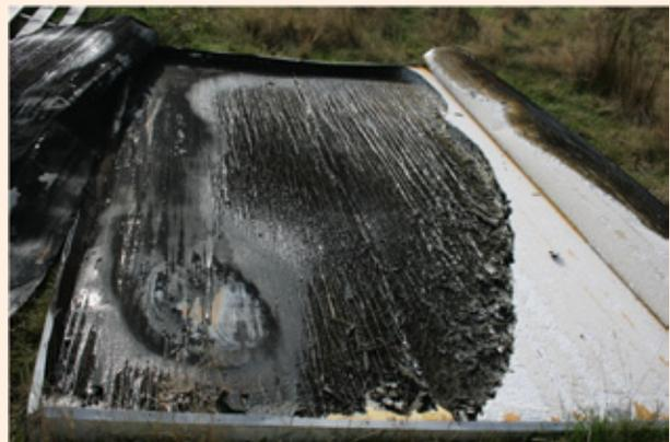
Figure 4: This is the Panel after exposure to the fire flame. The Panel core EPS-FR melts and runs away but does not continue to burn once the source of the fire is taken away. This testing has been repeated at BRANZ 2010 and at the NSW Fire Bridage 2011 with similar outcomes.
