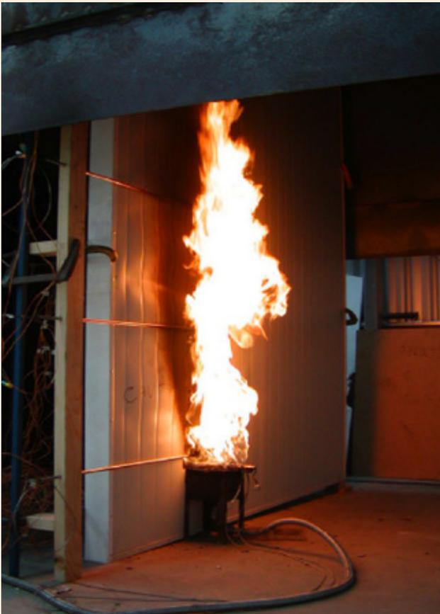
Figure 2: The experimental program was based on confirming work carried out by BRANZ in 2003 focussed on reviewing how to improve the performance of EPS-FR cored Panel in fire situations and firstly looked to review what actually happens when the EPS-FR core is directly exposed to flames, so a hole was cut in Panel, then a gas burner was placed up against the Panel.
