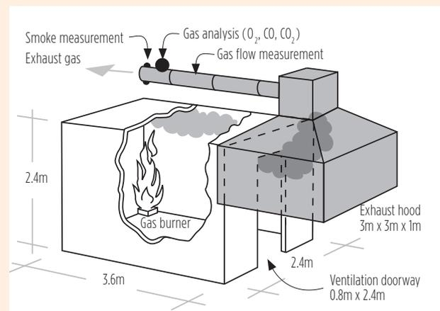
Figure 5: ISO 9705 Room Test (source<sup>10</sup>)
