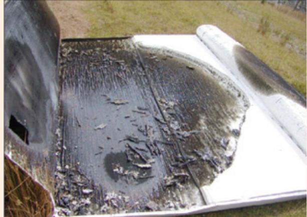
Figure 3: Result of 2003 tests at BRANZ – Note that there is no flame spread beyond where the flame has impinged.
