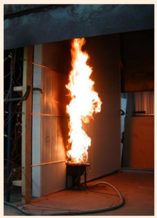
Figure 2: The experimental program was based on confirming work carried out by BRANZ in 2003 focussed on reviewing how to improve the performance of EPS-FR cored Panel in fire situations and firstly looked to review what actually happens when the EPS-FR core is directly exposed to flames, so a hole was cut in Panel, then a gas burner was placed up against the Panel.
