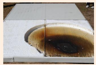
Figure 5: A demonstration burn at the NSW Fire Brigade facilities at Londonderry in 2011 replicating the BRANZ test results.
