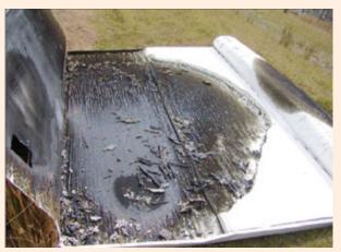
*Figure 3: Result of 2003 tests at BRANZ – Note that there is no flame spread beyond where the flame has impinged.*
