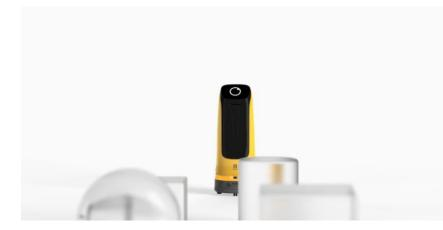
Powered by PUDU Slam algorithm, KettyBot supports laser slam and visual slam dual solution simultaneously in order to adapt to more scenarios. 2\* RGBD depth camera, provide KettyBot with the strongest 3D perception.
