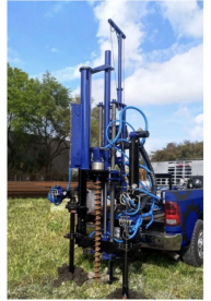
MB-23 Rotary Drill with depth capacity of 50 - 75 feet.
