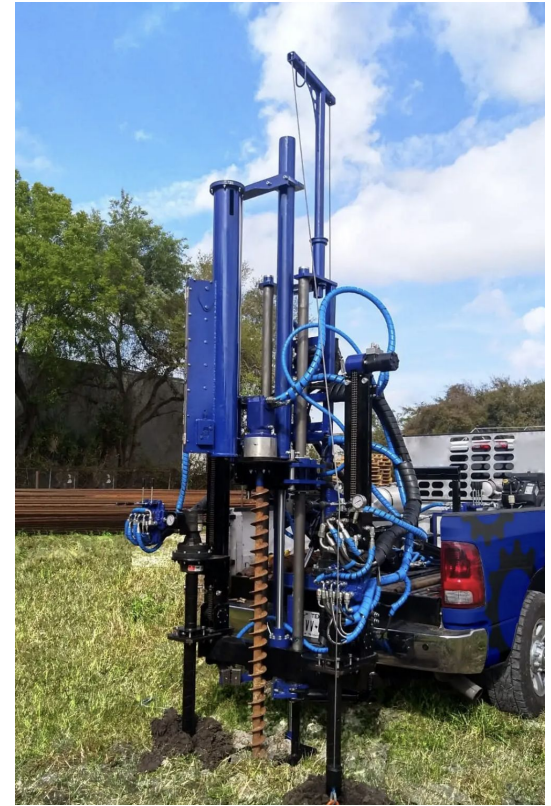
MB-23 Rotary Drill with depth capacity of 50 - 75 feet.
