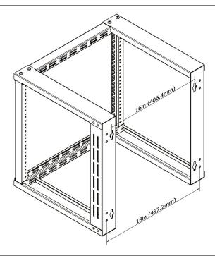
Attach the rack to a wall or other suitable mounting surface using M6 Wall Mounting Screws and M6 Metal Washers (Bag D). Mounting holes are spaced 16" (406.4mm) apart to accommodate standard stud placement as reflected in the diagram.
