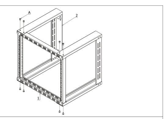
Attach Front Frame (#1) to the Side Frames (#2) and secure them with 8 of the M6 Installation Screws (Bag A).
