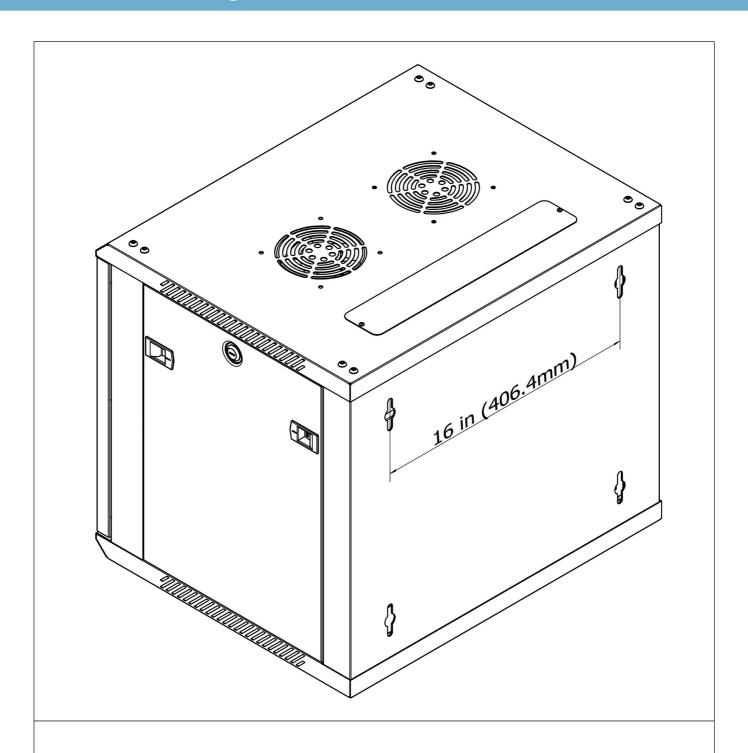
1: Attach the rack to a wall or other suitable mounting surface using M6 Wall Mounting Screws and M6 Metal Washers (Bag H). Mounting holes are spaced 16" (406.4mm) apart to accommodate standard stud placement as reflected in the diagram.
