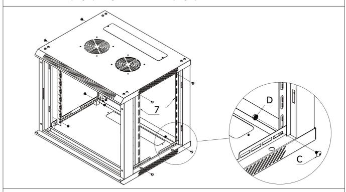
3: Install the 4 Vertical Mounting Rails (#7) into place at the desired depth using 2 M5 Screws (Bag C) and 2 black M5 Nuts (Bag D) for each Vertical Mounting Rails (#7).
