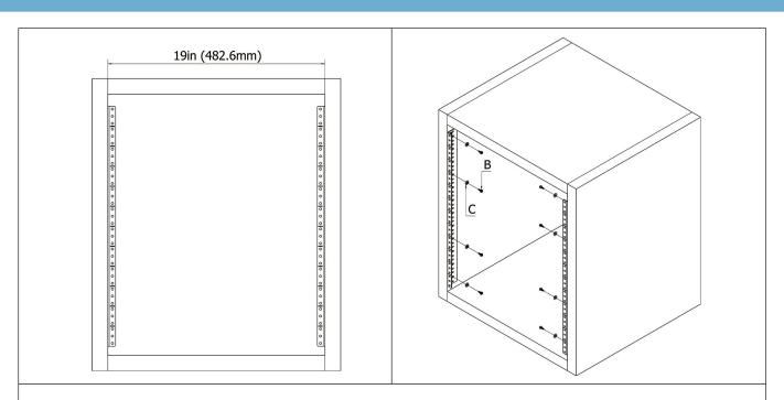
Attach the Vertical Rack Rails to the wood frame or other suitable mounting surface using M6 Rail Installation Screws (B) and M6 Metal Washers (C), make sure both Vertical Rack Rails are at same height.
