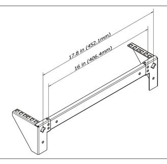
Attach the rack to a wall or other suitable mounting surface using M6 Wall Mounting Screws and M6 Metal Washers (included). Mounting holes are spaced 16" (406.4mm) apart to accommodate standard stud placement as reflected in the diagram.
