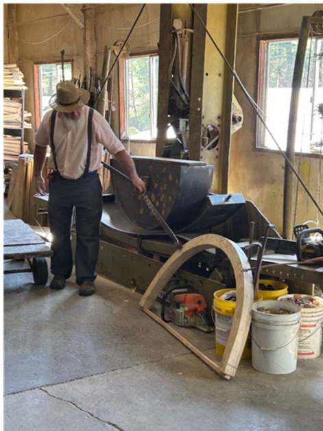
Demonstrating the use of a custom press used to bend wood into shape at Stutsman Wheel
