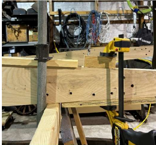
Drilling front suspension bolt holes using square guide block
