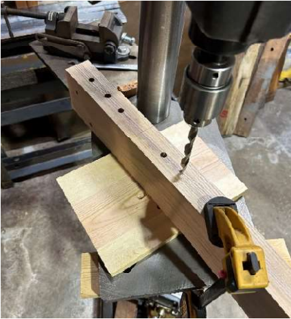
Drilling rear spring assembly mounting bracket holes
