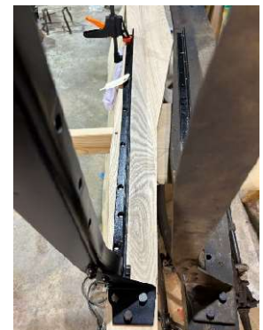
Fitting engine mounting brackets on the frame rail before marking and drilling eleven #20 wood screw holes (comparing to the original setup)
