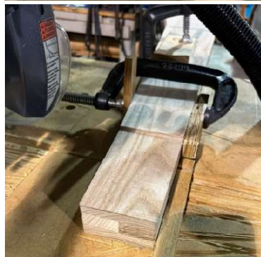
For the last pass with the dado blade, I braced the end of the cut with a piece of scrap plywood to prevent splintering.
