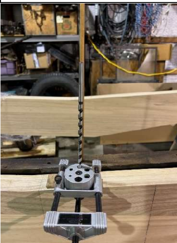
Drilling 5/16" diameter holes through the center of the frame rail
