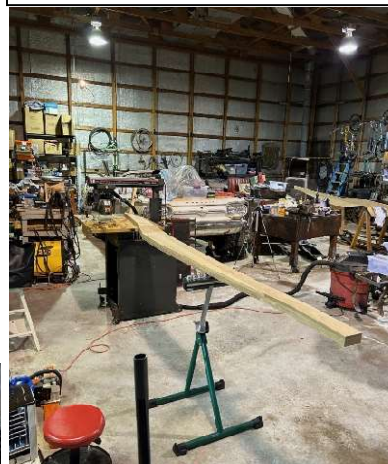
Supporting the frame rail while cutting with the dado blade (left (driver's) side frame rail)
