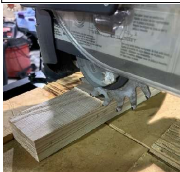
Milling off 1/8" of wood with a dado blade on the radial arm saw.
