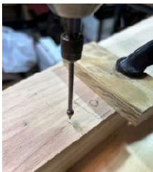
Finding a hole center before drilling one of the three holes for the front engine mounting bracket
