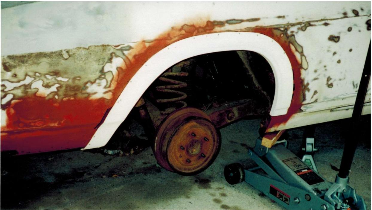
Front dog leg and door pillar area with metal panel patches welded in (red primer area) 2001
