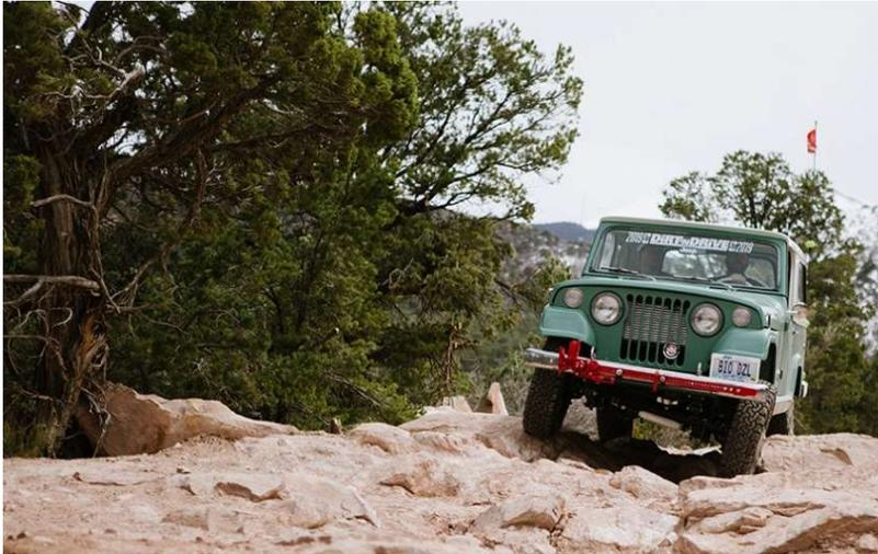
The Jeepster Commando was introduced by Kaiser Jeep in 1966 as a competitor to the International Scout and Ford Bronco, both of which offered more civilized comforts relative to the Jeep CJ5. The Commando uses the same drive components as a CJ5 and the same chassis as the longer (101”) wheelbase CJ6.
