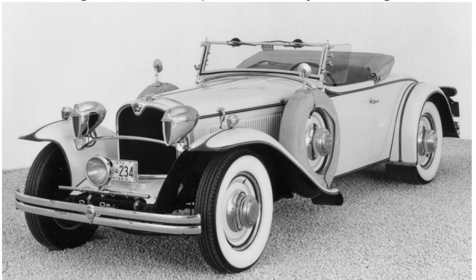
concentrate and project a beam of light farther down the road than a conventional headlight. You can read Wood's description of the method of operation, and check out diagrams of the Woodlite's interior geometry, in the U.S. patent granted July 31, 1928. Wood filed a series of patents for headlights, and the one that outlined the ornamental appearance of the Woodlite can be read here
