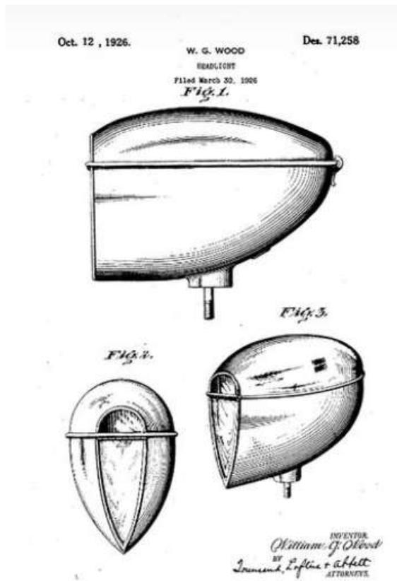
The patent filing for the Woodlite's ornamental appearance. A separate patent details the theoretical operation of the headlight design, which was intended to focus and project light farther down the road than a conventional unit.
