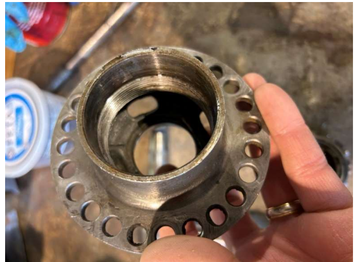
Caption: Steering gear bearing housing after cleaning. The multiple holes are drilled on an eccentric housing to allow for gear lash adjustment. Move the housing clockwise/counter clockwise relative to the steering box brings the steering gear and pinion gear closer together or further apart.
