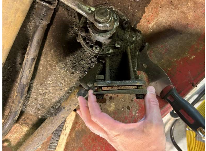
Caption: Drive shaft coupling and pinion gear housing. Note safety wire lacing bolts. Many bolts are drilled for safety wire on this car.
