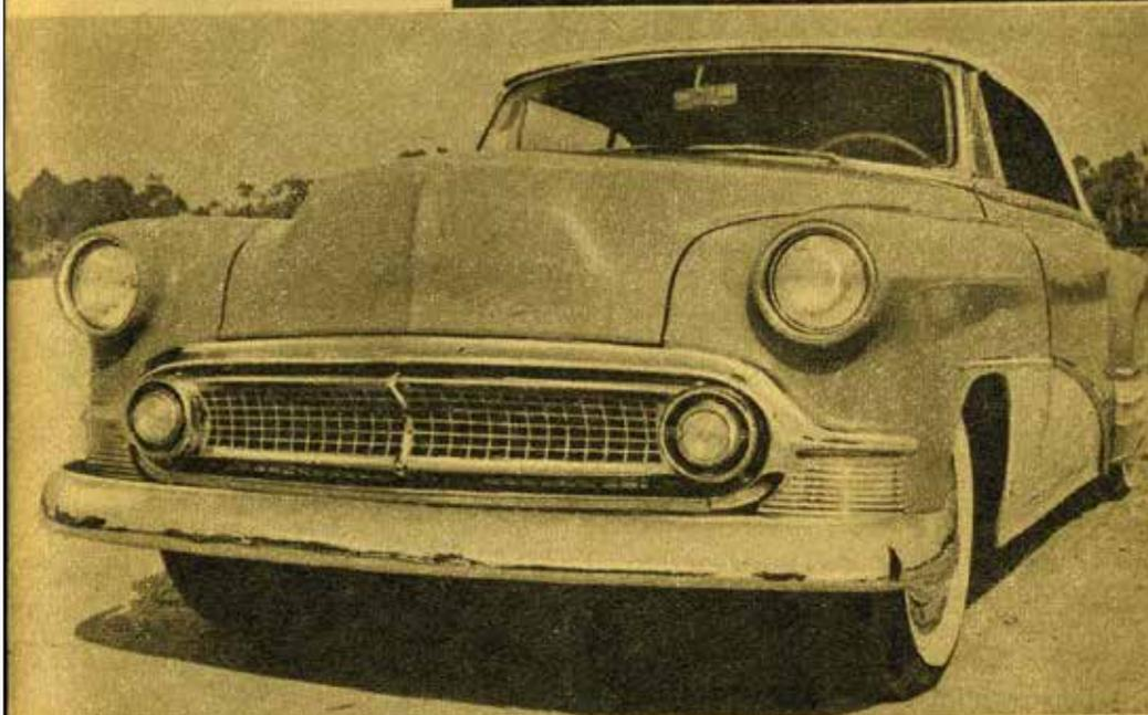
'55 Ford grille center section was neatly spliced into stock Chev parking lights. Trimless hood has been slightly peaked. Front bumper bolt holes have been eliminated (see page 40) for trim appearance.
