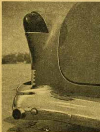
Headlights have been frenched to fenders, utilizing '53 Ford deeply tunneled headlight rims. Large '54 Packard taillights have replaced the stock blinkers. Small diameter welding rod was used to create edge of taillight's openings. Sheet metal was employed to fill in extended areas. Exhaust tips have been routed out through '51 Oldsmobile rear bumper. Deck lid and doors are absent handles and now operated by an electrical push button system.
