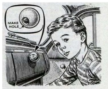
Ball Protects Children. Knobs or handles on the dash can give youngsters a bad bump on sudden stops. Sponge-rubber balls fitted over the protruding parts reduce this hazard. A dab of gasket shellac in the hole will attach the ball securely.
