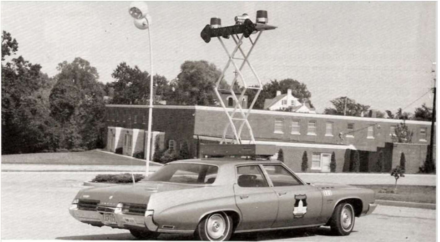
One of two vehicles received from the National Highway Safety Act. Seen is a 1971 Buick, equipped with an elevated traffic and warning bar. Photo courtesy: JCPD
