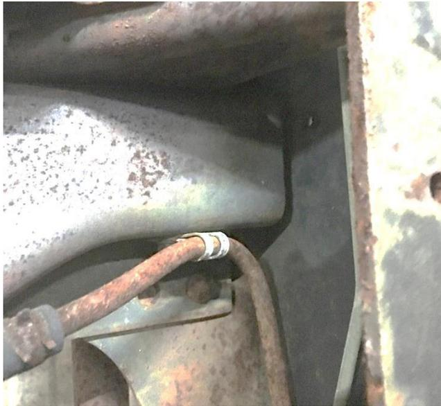
DRIVERS SIDE – Note two bolts are on back side under mount and 2<sup>nd</sup> rivet is hidden under mount. It will be visible after mount is removed.
