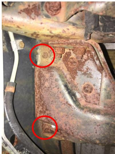
PASSENGERS SIDE – Remove two bolts attaching to mount.
