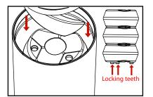
6. Once the Blast Pack™ ice packs are frozen, place them back into the Breeze Blast™ base. For best results, install the Blast Pack™ ice packs with the locking teeth facing downwards. Install lid by turning clockwise onto base.
