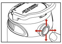
8. The Breeze Blast<sup>™</sup> lid has a built-in, multi-directional eyeball valve. To use the eyeball valve, use your index finger to rotate nozzle in the desired direction of air flow.
