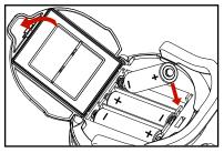
**1. SETUP** Requires (3) AA batteries installed as shown (not included). Open battery compartment by lifting on the locking tab. For best results, install new alkaline AA batteries. DO NOT mix battery types.
