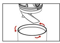
1. Rotate Breeze Blast<sup>™</sup> lid counterclockwise to remove lid from body. Clean Breeze Blast<sup>™</sup> base with a warm damp towel. DO NOT WASH IN DISHWASHER.
