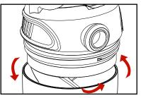
2. Twist off Breeze Blast<sup>™</sup> lid counter clockwise to remove cap from Breeze Blast<sup>™</sup> base.
