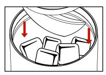
Optional cooling: The Breeze Blast™ cooling system works with ice as well. Add 2 cups of ice cubes (maximum). Remove excess ice if lid does not tighten properly. For best results, remove lid, pour out melted ice water, and replace ice as needed.
