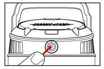
Press the power button to turn on the system. Press power button again to turn system off. Auto shut-off timer turns unit off after 30 min. Simply push power button to reactivate air flow.
