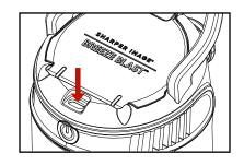
Optional USB power method: To power the device directly, connect a micro-USB power cord (included) into any USB powered port such as a computer, phone charger, or battery bank. Use of power cord does not charge reusable batteries.
