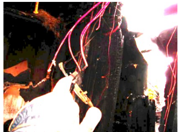
(b) Actual fire origin at branch circuit wiring inside the wall (note beading)
