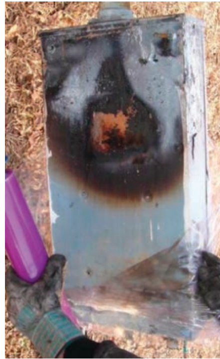
(b) Burn patterns on back of housing
