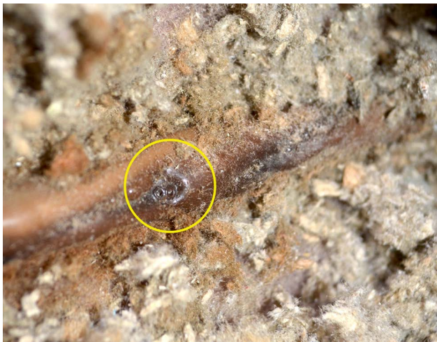
Figure 81 A damaged section from a cable in the same fire as shown in the previous figure. Note that there is no fire damage here, but a severe, localized insulation failure. The two dimples (in the middle of the yellow circle) are not mechanical damage. There was no mechanical damage, but evidently the cratering of the insulation occurred due to localized damage from RF waves. This location was about 2 m away from the smart meter. (Photo: Jim Brown)
