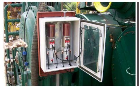
(above left) Hydromatic Brake Automatic re-lubrication of multiple bearings. Utilizing the perma PRO MP-6 all bearings receive controlled, uncontaminated lubrication on a consistant basis.
