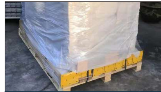
Palletizing properly to reduce abrasion during transportation
