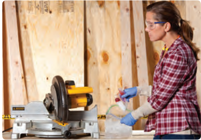
Figure 10-16. Wrap a severed body part in sterile gauze, place it in a sealable plastic bag, and put the bag in an ice and water slurry.
