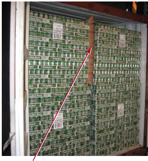
This picture shows an air bag stabilizing a container load
