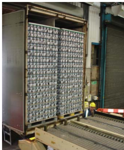
Unloading by live bed conveyors at customer
