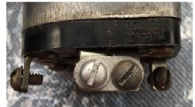
Jumper between terminal "R" and adjacent GND. TCM p/n 10-126656
