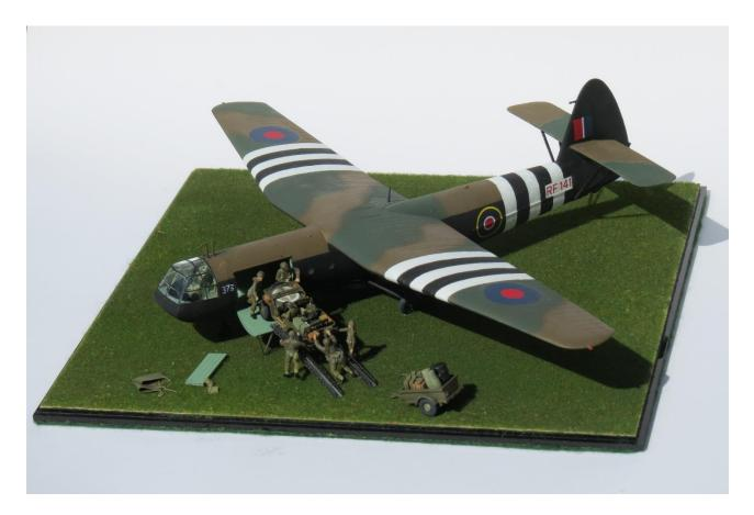
On landing in France, the tail section of the glider was removed, and the gutters placed so that the Jeep could be easily driven out of the rear of the aircraft. Later, for Operation Varsity in 1945, the Rhine crossing, the Mk II Horsa had a side hinged nose section, which made the loading easier, when the Jeep could be driven straight into the fuselage from the front.
