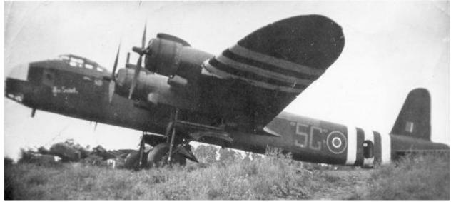
Originally designed as a bomber and specified to drop large numbers of smaller bombs (maximum bomb size 2000 lb) due to the bomb bay construction, and having a height limitation (a service ceiling of 16,500 ft) the Stirling was soon relegated to other duties, when Lancasters and Halifaxes, which flew higher and had a longer range with larger bombs, became available in large numbers.
