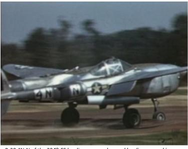
P-38 4N-N of the 394<sup>th</sup> FS landing on an advanced landing ground in France. The tar paper is ballooning in front of the main landing gear like it was described by Ernie Snow, the propeller specialist of the squadron. These pictures come from TV news of summer 1944 and it could have been filmed at ALG A-44 because of the tar paper.
